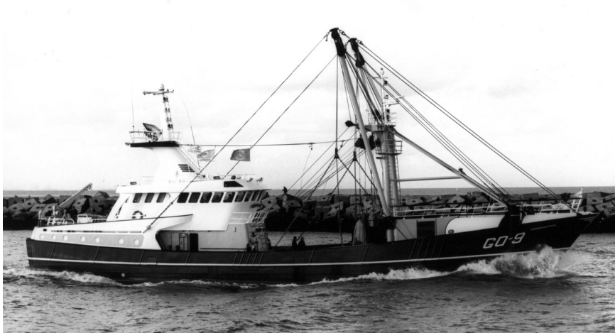
Figure 3. Beam trawler with closed poop Building year: 2002 Size: 471 GT Length: 41 m. Power: 2000 HP
