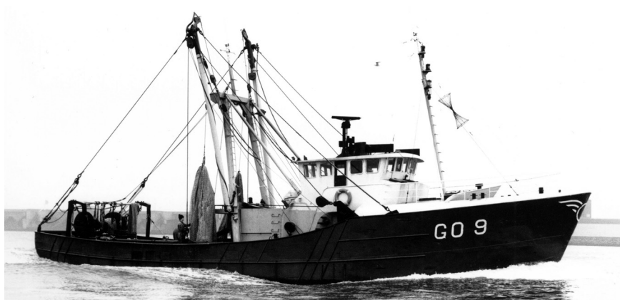
Figure 1. Beam trawler with free standing deck house Building year: 1967 Size: 107 BRT Length: 26 m. Power: 680 HP
