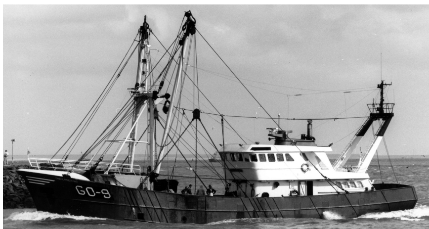
Figure 2. Beam trawler with open poop Building year: 1984 Size: 301 GT Length: 36 m. Power: 2180 HP
